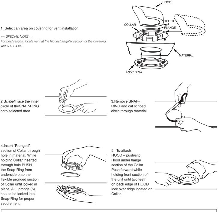
For trailer type covers, point the Hood opening opposite to the direction of towing vehicle during travel for best venting effect. TO REMOVE HOOD, press down on front section of HOOD to lift two teeth on back edge over sharp ridge – slide HOOD off.
