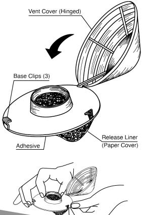
1. Select an area on covering for ventilator installation.
