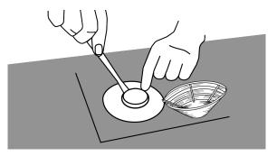
3. Cut through covering material at the center of the vent, and remove all covering material from the center of Vent opening.
