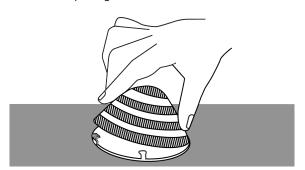
5. Lock vent COVER onto BASE by pressing COVER down firmly onto BASE until all (3) Base-Clips are firmly attached over flanged area of vent cover.
