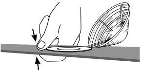
4. Press vent firmly into place by applying finger pressure to both sides of BASE perimeter.
