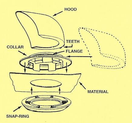
For trailer type covers, point the <u>Hood opening</u> opposite to the direction of towing vehicle during travel for best venting effect.
